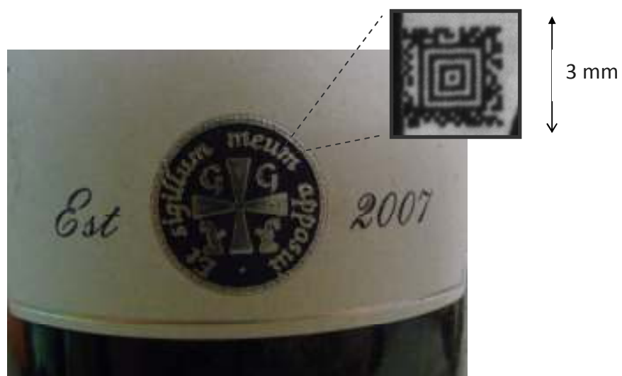
A 3x3 mm 2 EN-TAG™ on a wine label for thermal monitoring and authentication applications
